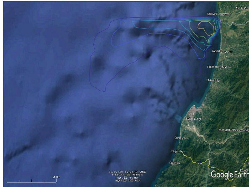
Figure 94: Result of west wind condition for Choruhi River
