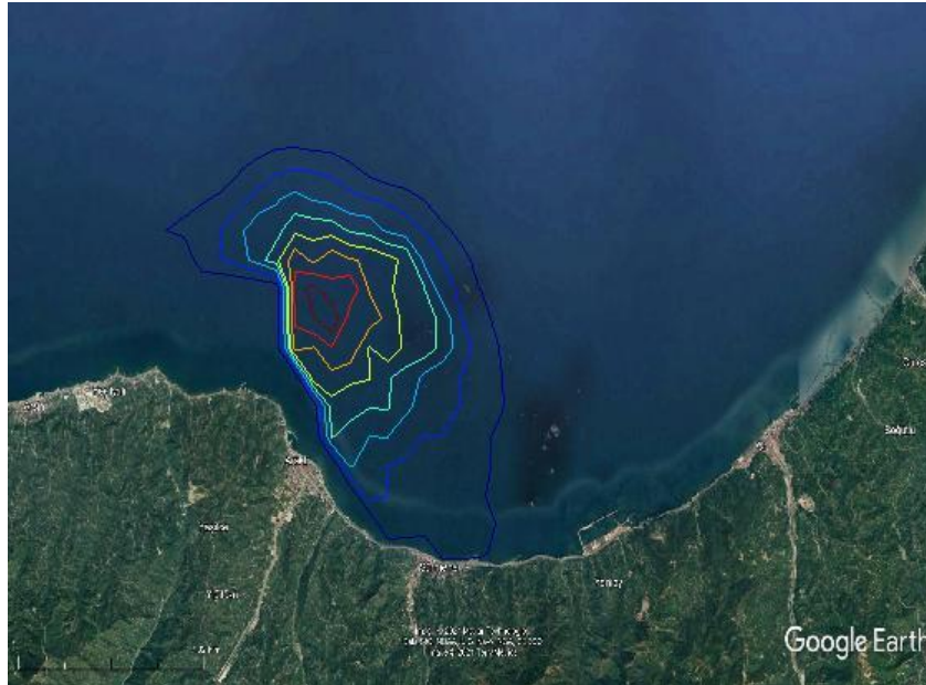
Figure 33: Result of Northeast wind condition for Sürmene River
