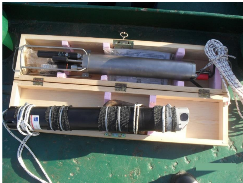
Figure 13: CTD and current meter used in the sampling provided by the Project coordinator
