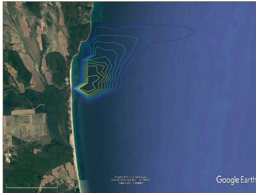
Figure 52: Result of East wind condition for Kamchia River
